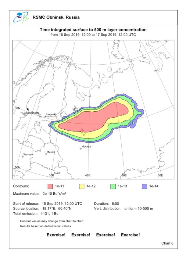
Figure 7. Second 24-hour average exposure forecast for a hypothetical accident
