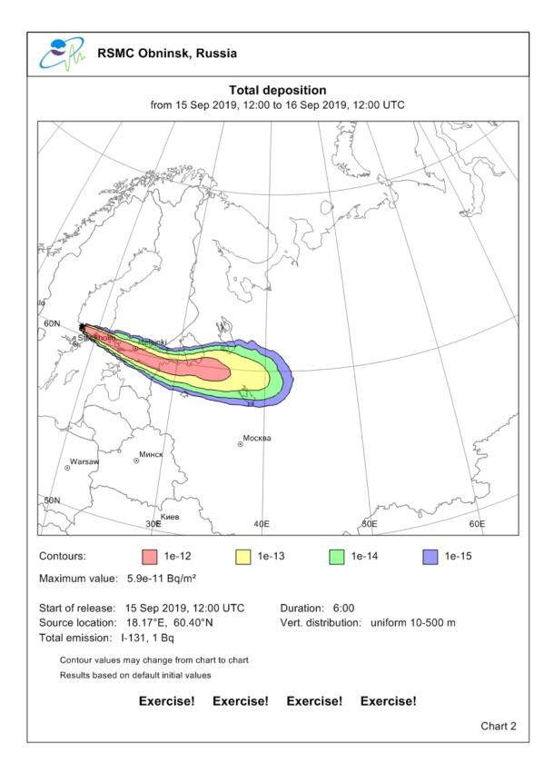
Figure 3. 24-hour total deposition forecast for a hypothetical accident
