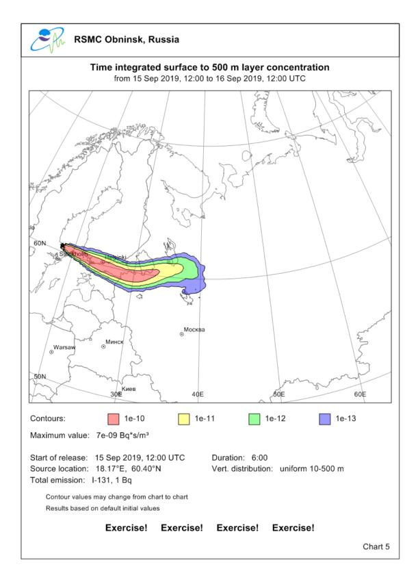
Figure 6. First 24-hour average exposure forecast for a hypothetical accident
