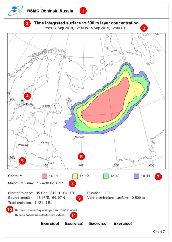
Figure 8. Third 24-hour average exposure forecast for a hypothetical accident. The red circled numbers are for reference in this document only and do not appear on the forecast products.
