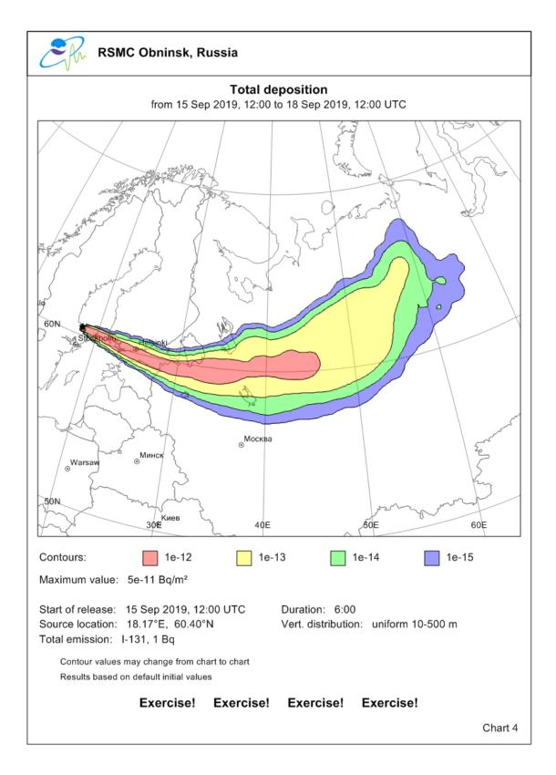
Figure 5. 72-hour total deposition forecast for a hypothetical accident
